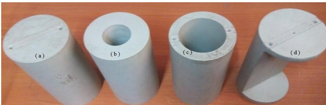
**Figure 5: Phantoms of Perspex Material, (a) Full Cross Section (b) Large Annular Ring of PM (c) Small Annular Ring of PM (d) Half Cross Section (Stratified)**
