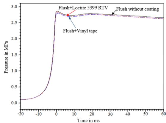
Figure 7: Air pressure traces using transducer 701A flush mounted, with and without coatings
