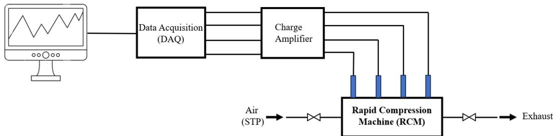
**Figure 3: Experimental setup for simultaneous pressure measurements in RCM.**
