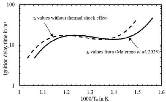
**Figure 1: Effect of pressure error due to thermal shock on ignition delay times ( $\tau_i$ ) curves.**
