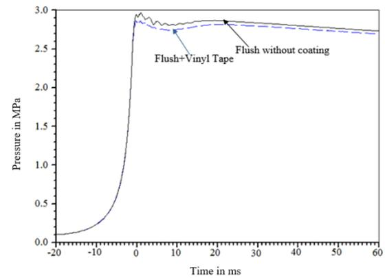
Figure 6: Air pressure traces using transducer 6061B flush mounted, with and without coatings.
