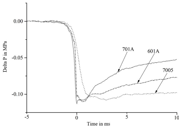
**Figure 4: Magnitude of thermal shock error for different pressure transducers.**
