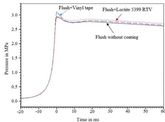
Figure 8: Air pressure traces using transducer 7005 flush mounted, with and without coatings
