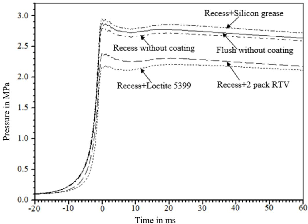
Figure 9: Air pressure traces using transducer 601A when recess mounted with and without coating, and when flush mounted without coating.
