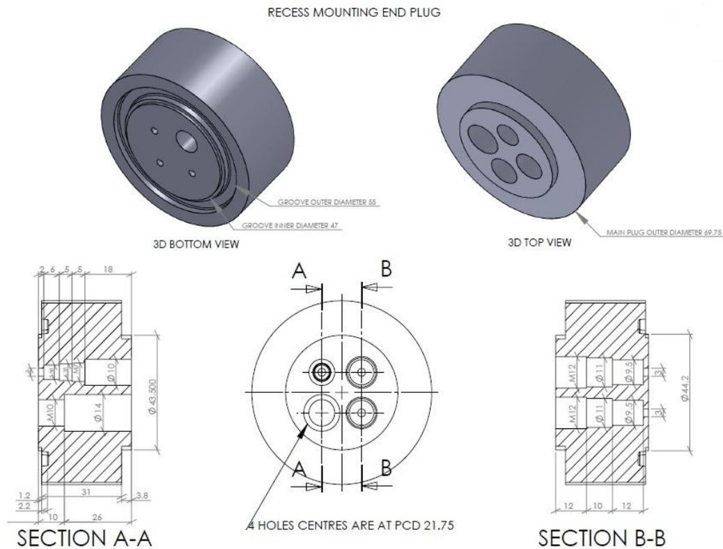
**Figure 2: End plug for recess mounted pressure transducers.**
