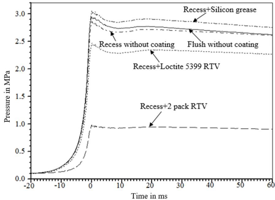
Figure 10: Air pressure traces using transducer 7005 when recess mounted with and without coating, and when flush mounted without coating.
