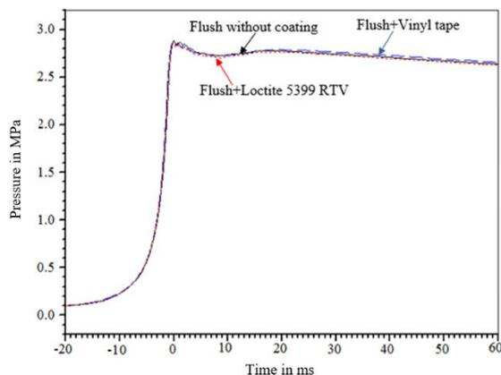
Figure 5: Air pressure traces using transducer 601A flush mounted, with and without coatings
