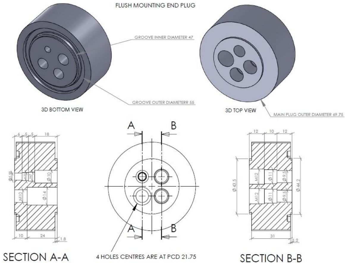
**Figure 1: End plug for flush mount pressure transducers.**
