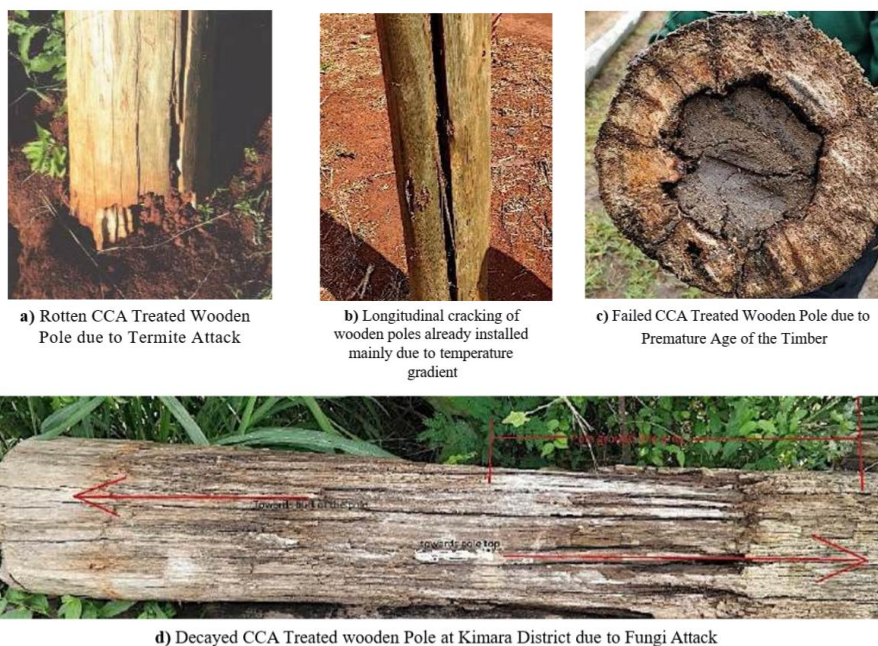
Figure 8: Pictorial presentation of different reasons for early rotting of CCA treated wooden poles in Tanzania.
