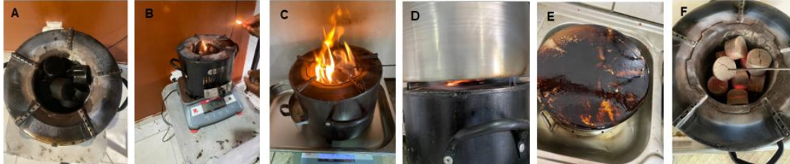
Figure 10: Images of combustion: A) Briquettes soaked in paraffin in the combustor; B) Ignition of the paraffin; C) Ignition of the briquettes; D) Emission of white smoke during boiling; E) Adherence of brownish oil in the pan; F) Formation of ash around the briquettes.
