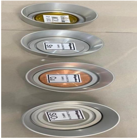
Figure 1: Calibration of EDXRF machine using MCA calibration samples.
