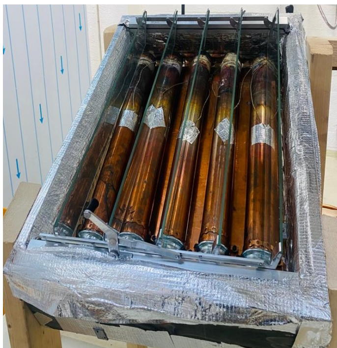
Figure 2: Adsorber bed for ARS integrated with glass louvers
