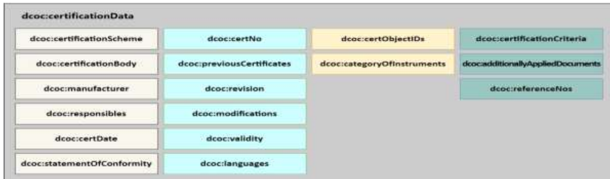
Figure 6. Overview of the basic sub-elements within the root element of administrative data (dcoc:certification Data)
