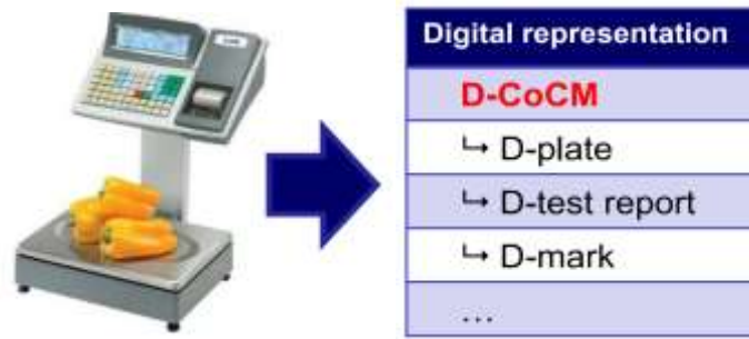
Figure 3. Digital representation of certificate of conformity of legal measuring instrument
