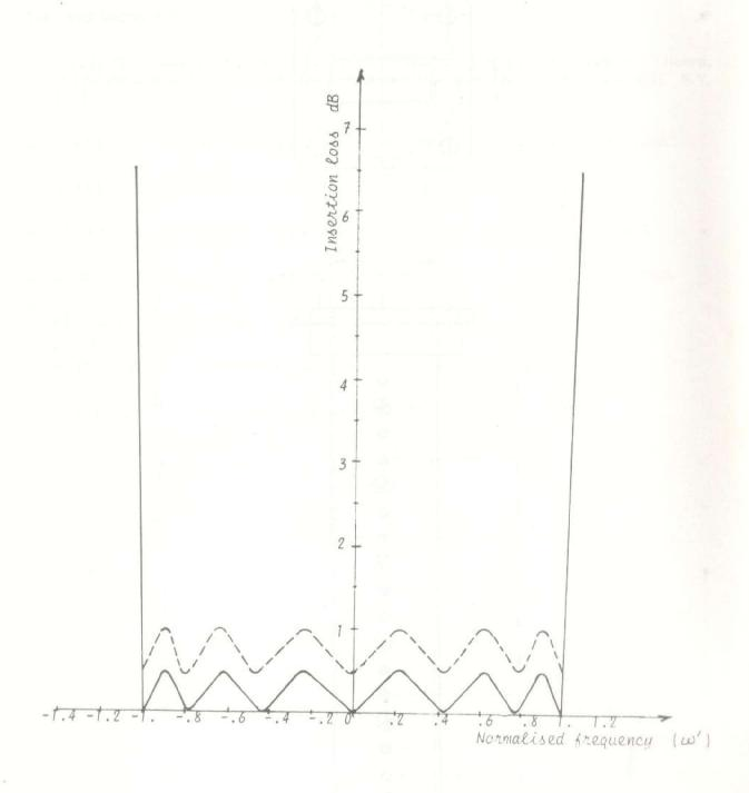
Fig. 2 Measured ( dashed curve ) and theoretical ( solid curve ) INSERTION LOSS CHARACTERISTICS of the seven stage filter
