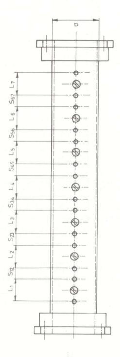
Fig.1: Designed seven stage wave guide filter.
