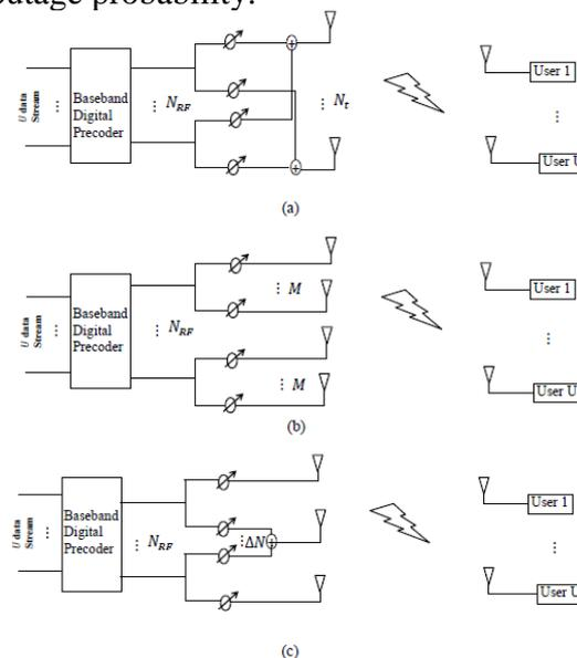
**Figure 1: Hybrid beamforming architectures (a) Fully array architecture, (b) Sub array architecture, and (c) Overlapped sub-array architecture.**
