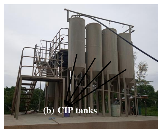
Figure 14: (a) Ball mill (b) CIP tanks at Itumbi mineral demonstration centre.
