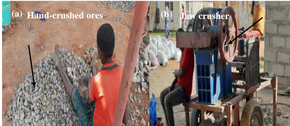
Figure 7: (a) Hand crushing (b) Jaw crushing operations at Nholi gold mine, Dodoma.
