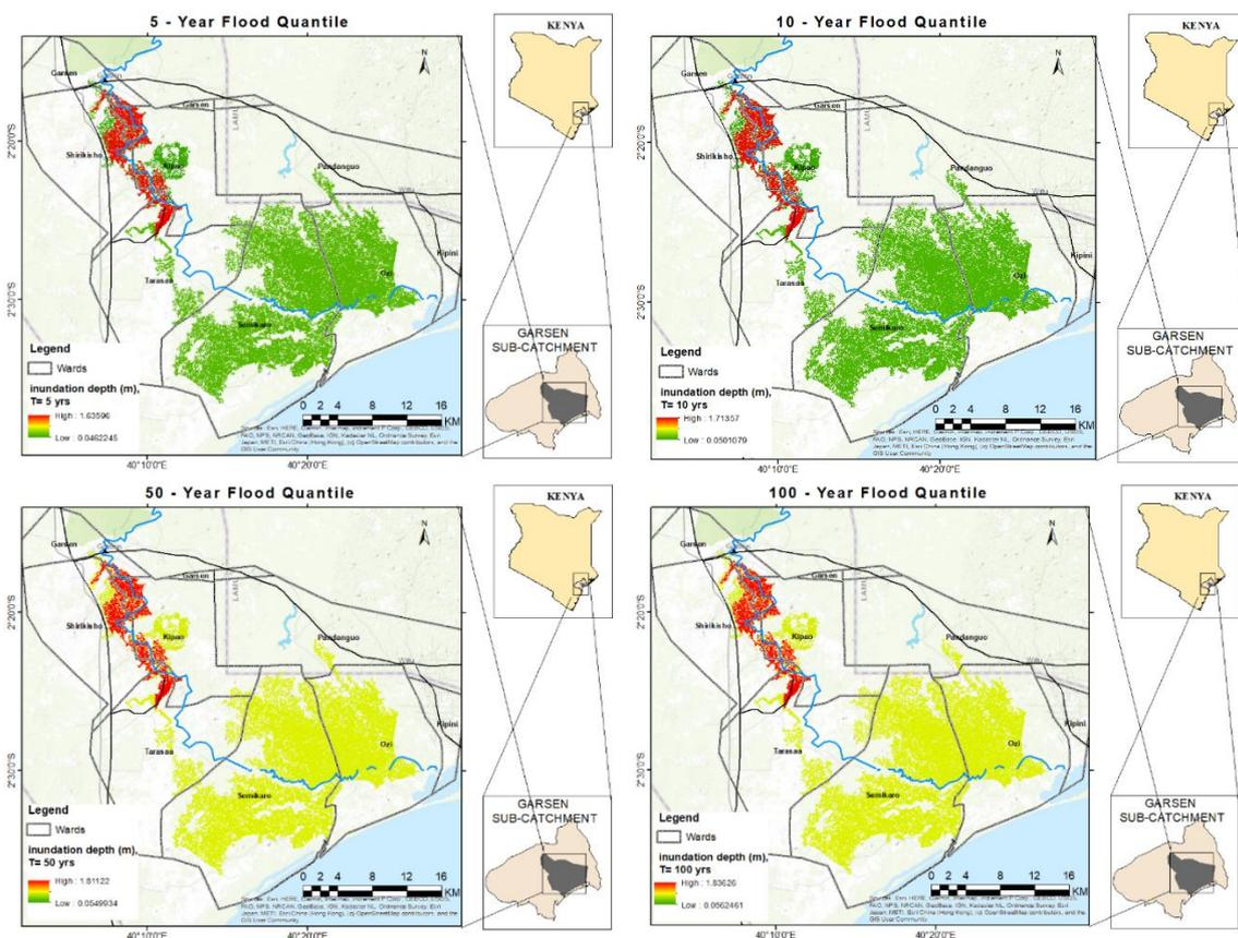
Figure 4: Inundation extent for different flood quantiles.
